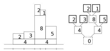
Figure 7.5: Illustration of the k-split algorithm, k=2. The numbers in boxes represent the observation count values
