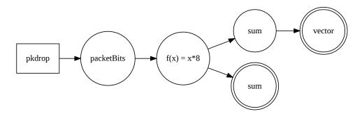
Figure 4.4: Result filters and recorders chained
