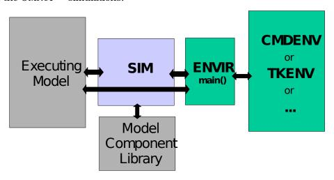
Figure 18.1: Architecture of OMNeT++ simulation programs
