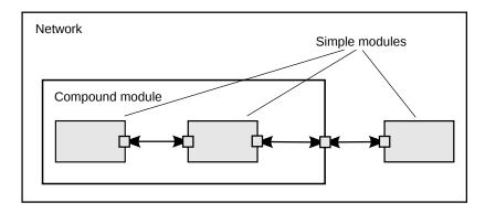
Figure 2.1: Simple and compound modules
