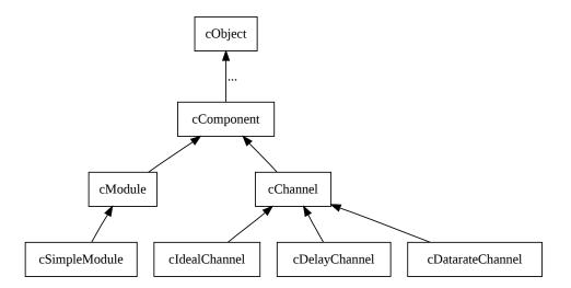
Figure 4.1: Inheritance of component, module and channel classes
