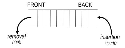
Figure 7.1: cQueue: insertion and removal
