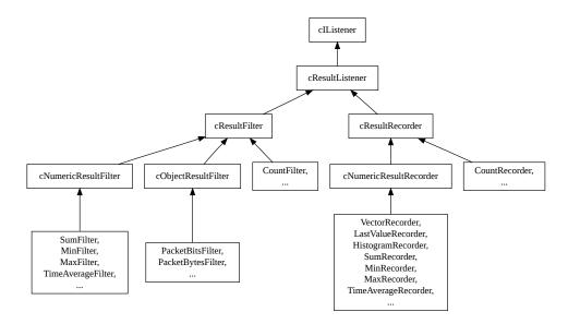
Figure 4.5: Inheritance of result filter and recorder classes
